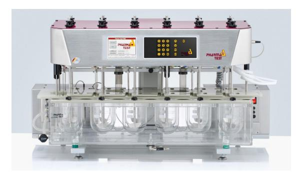
The PTWS D620 is a "Dual Drive" 6 + 6 position, single drive tablet dissolution testing instrument for solid dosage forms as described in USP chapter <711/724> and EP section<2.9.3/4> as well as the DAB/BP and Japanese Pharmacopeia section <15>. The instrument features two additional vessels (approx. 250ml) for media refilling and reference standard media. PTWS D620 features independent stirrer speed control for the front and back row of stirrers.
